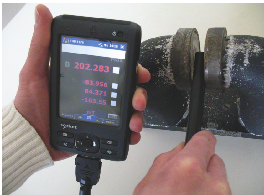
Figure 7 This three-axis Metrolab probe has USB output and comes with an optional PDA (courtesy GMW Associates).
