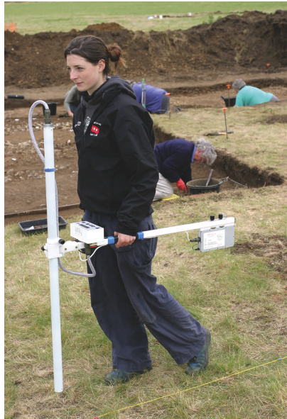
Figure 2 This field researcher is using a Grad601 flux-gate gradiometer at an archeological-dig site (courtesy Bartington).
